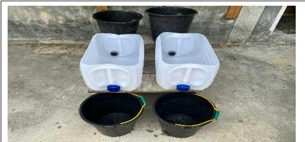
Gambar 3.5 Media *Constructed Wetlands* (CWs) dengan sistem *sub surface flow*
