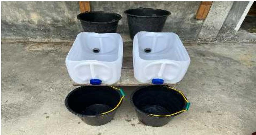
**Gambar A.6 Media *Constructed Wetlands* (CWS) dengan sistem *sub surface flow***
