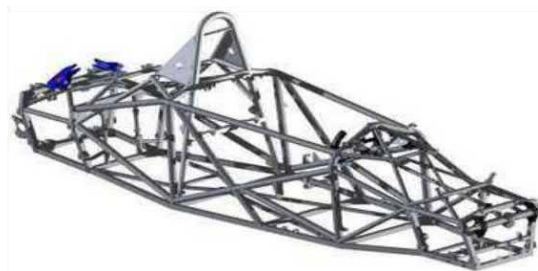
Gambar 2.6 Tubular Space Frame (Sumber: Nur Arifin, 2019)
