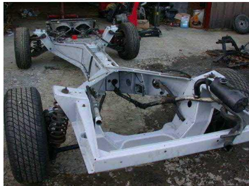
Gambar 2.8 Chassis Backbone (Sumber: Nur Arifin, 2019)
