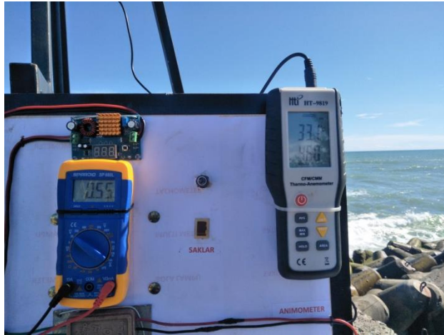
Gambar B.4 Pengambilan Data Turbin Angin (Sumber: Penelitian)
