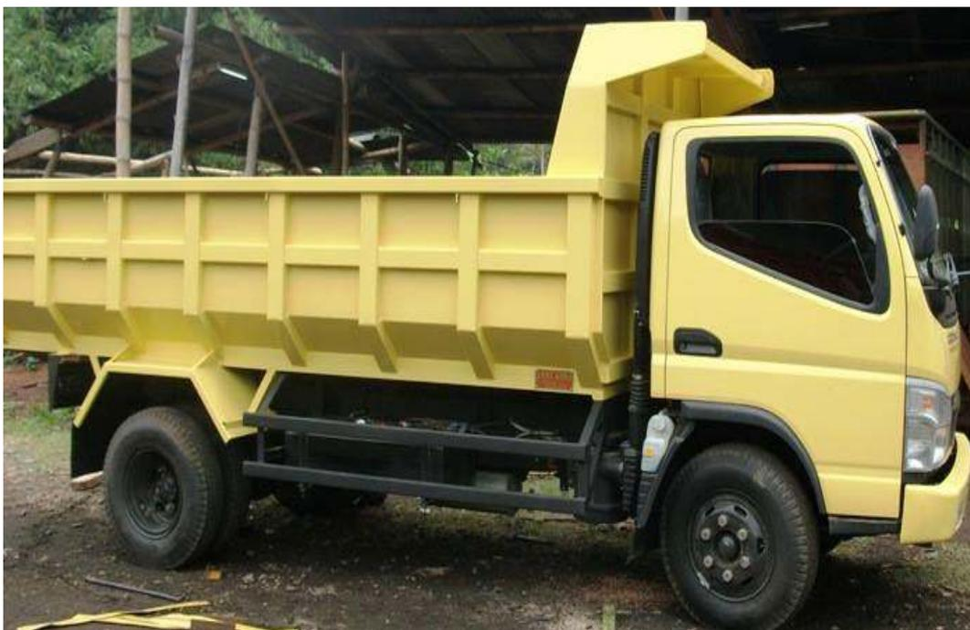
**Gambar 2.5.** *Dump Truck* Kapasitas Muatan 1 ton
