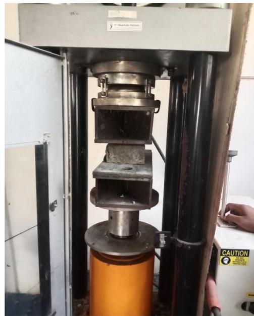
Pengujian kuat tekan *compression testing machine*
