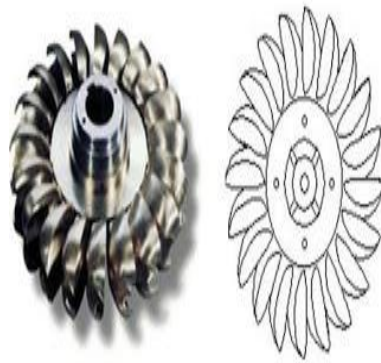
Gambar 2.2 Runner Turbin Pleton (sumber : Dwi Ratna, Turbin air. 2015)
