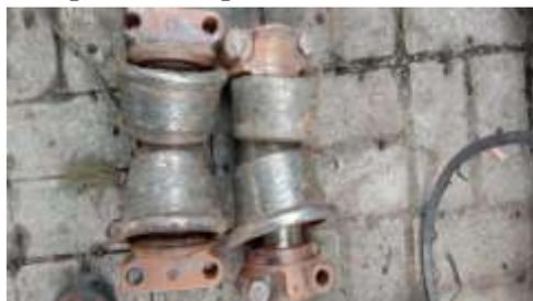
Gambar 3.7 Track Roller Mengalami Kehausan
