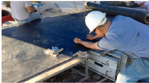
Gambar 2.3 Proses Pemotongan Belt Conveyor
