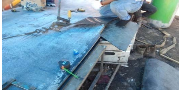
Gambar 2.4 Proses Pengupasan belt Coneyor
