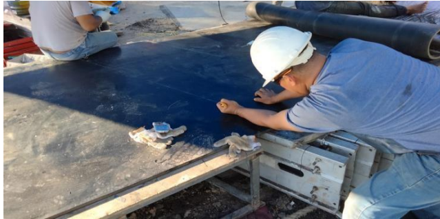
Gambar 5. Proses Pemotongan Belt Conveyor
