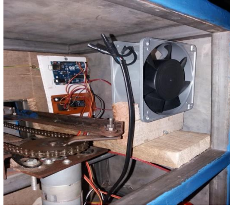
Gambar 4.5 Perakitan Tombol On/Off Kipas Pendingin
