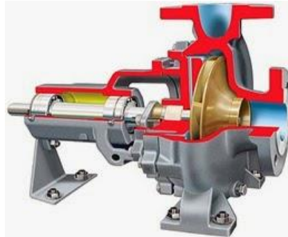
Gambar 2.6 Condensate Water Pump ( Sumber : konversienergi-haga.blogspot.com )
